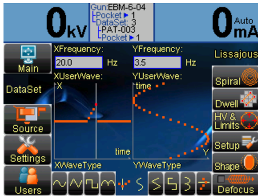
Fig. 9. The menu and the result of a Lissajous deflection
