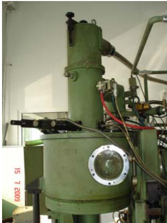
4. Fig. 5. The electron beam hardening equipment in the projected position of gun against the chamber
